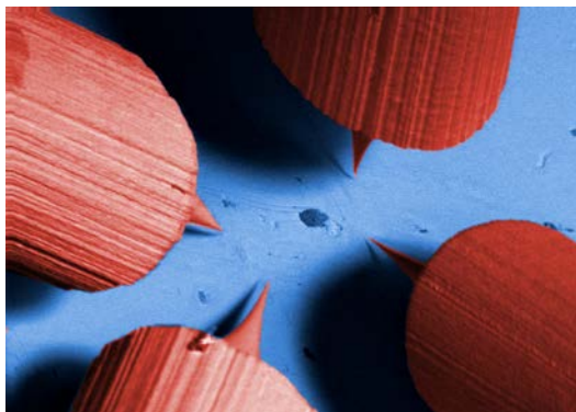
Fig. 2 SEM image of four tips (diameter 250 \mu\text{m} ) close to the surface. Imaging with the secondary electrons leads to a shadow effect giving access to the tip sample distance. The dark shadow of the tip is seen best for the lower left tip.
